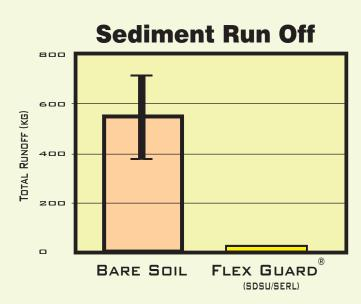
Mean total runoff volume and from the bare soil and Flex Guard<sup>®</sup> experiments with simulation variability shown as error bars.
