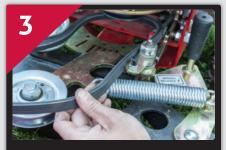
Slip the drive belt off of the engine, leaving the belt with the attachment. Each attachment includes its own belt.
