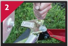
Remove the drive belt by releasing the tension lever. Some attachments include a pin to hold the tensioner open.
